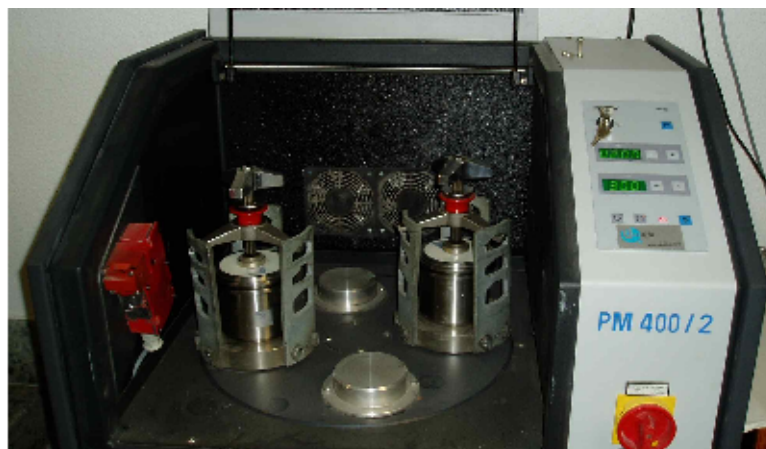
Figure 4.1: Planetary ball mill Retsch PM 400/2. WC balls and containers have been used in our particular case.
