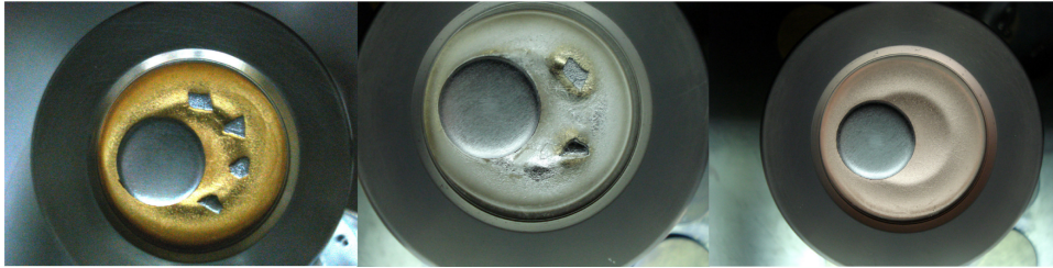
Figure 4.3: Targets used in the sputtering process. In the left panel the target for the evaporation of the Fe_7Au_{93} is shown. In the middle, the target for the Fe_{14}Ag_{86} and in the right the one for the Fe_9Cu_{91} samples. The final composition depends not only on the rate of noble metal/iron in the target but also on the different sputtering rates of the elements or the position of the Fe pieces.
